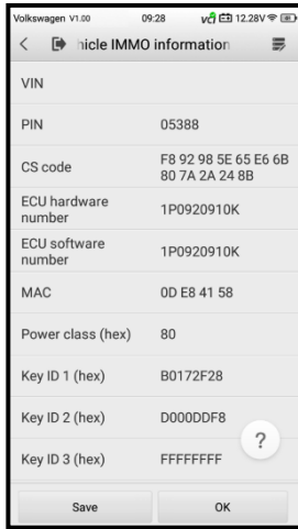
Figure 7-11 Vehicle IMMO Information Screen
